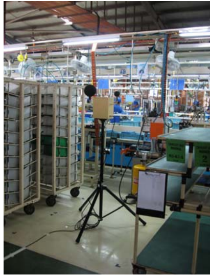
Figure 6: Environmental Monitoring Equipment and the Location Measurement.
