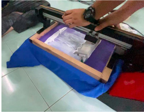
Figure 8. Slow squeegee movement cause ink blockage.
