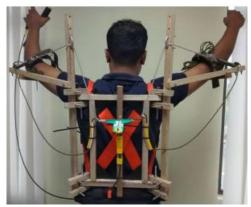
**Figure 4**. Study of passive exoskeleton for oil palm harvesting [17].
