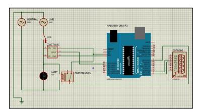
Figure 4. Hardware Connection Diagram by Proteus 8.
