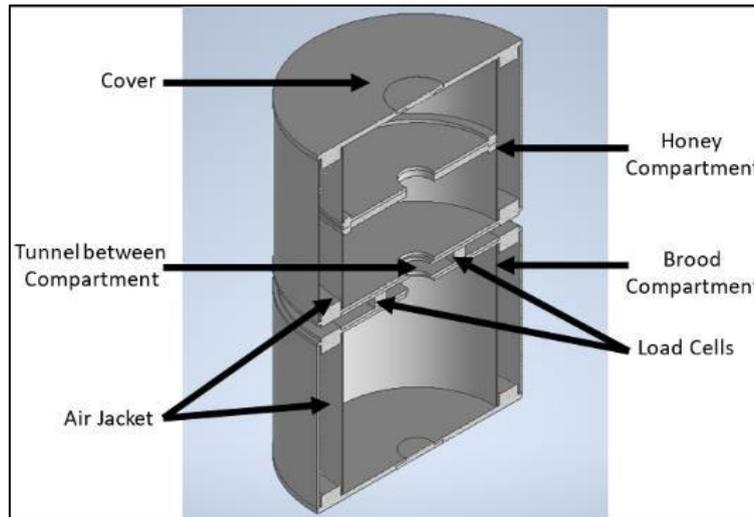
**Figure 1.** Drawing of Artificial Stingless Bee Hive
