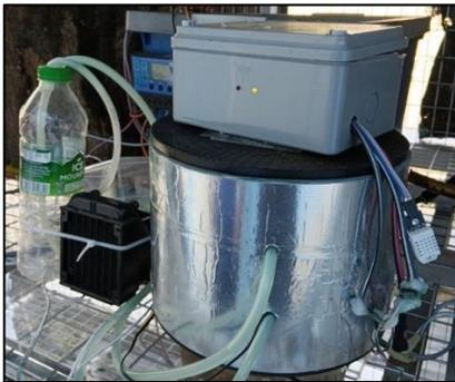
**Figure 8.** Artificial Hive with Water Cooling System
