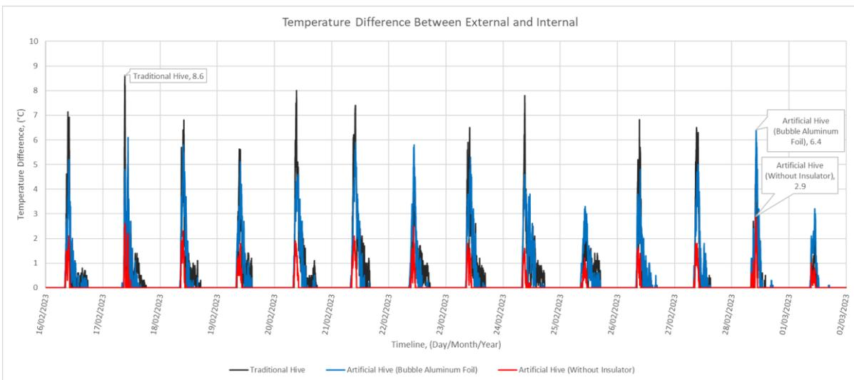
**Figure 10.** Graph of Temperature Difference Between External and Internal Artificial Hive Highlights for Traditional Hive, Artificial Hive (Bubble aluminium foil) and Artificial Hive without Insulator
