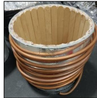
**Figure 9.** Copper Coil Pipe for Water Cooling System
