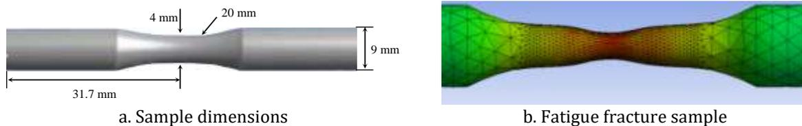
Figure 9. Fatigue sample mesh and stress distribution.
