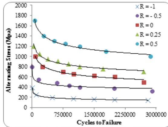
**Figure 17.** Influence of stress ratio on fatigue life characteristics (0% nano).
