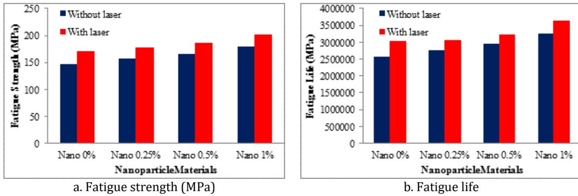
**Figure 14.** Fatigue strength and life for steel samples with nanoparticle and laser treatment effect.
