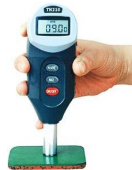
Figure 1 Hardness test (TH210 Shore Durometer)
