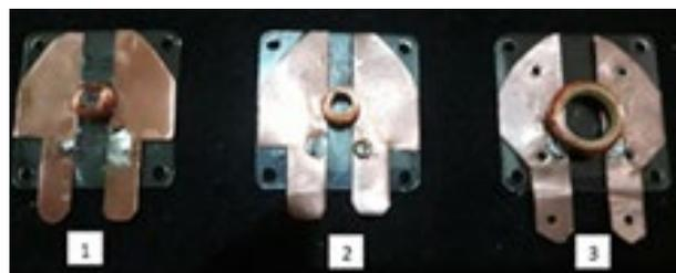
**Figure 5.** 3 Various coils formation (1), coil with air core (2), coil with large diameter (3).
