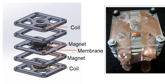
**Figure 4** Energy harvester with PDMS Membrane, (a) the schematic of the structure, (right) the photograph of the EM-VEH device.
