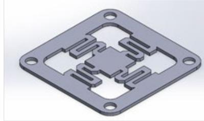
**Figure 1.** Design A: Spring arm membrane with a spring arm at the center of the membrane.
