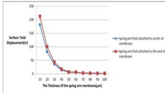
**Figure 3.** Effect of the membrane thickness on the mechanical deformation.
