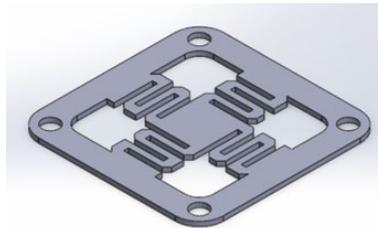
**Figure 2.** Design B: Membrane with a spring arm at the edge of the membrane.
