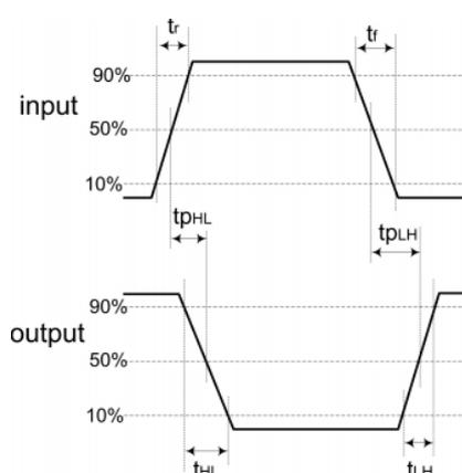
**Figure 2.** Calculation of the propagation delay of the circuit.
