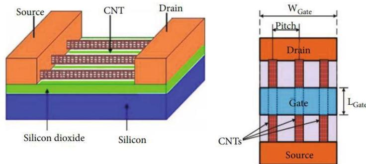
**Figure 1.** Carbon nanotube field effect transistor (CNFET). (a) Schematic. (b) Top view [15] Taguchi method.
