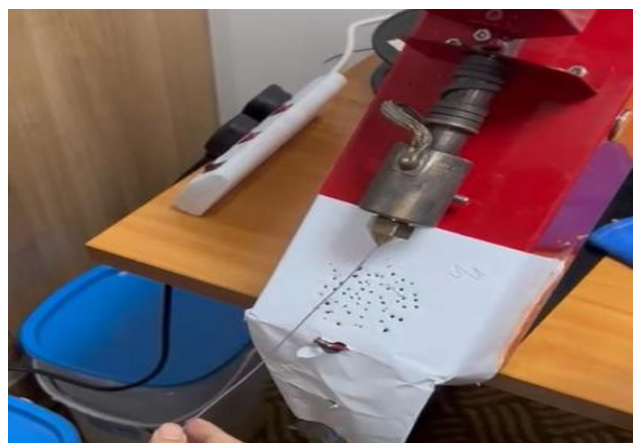
Figure 2. Extrusion process of PET-GNPs filament using a mechanical extruder.
