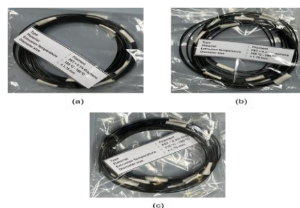
Figure 3. Fabricated PET-GNPs process and filament: (a) PET-0.1 wt.% C, (b) PET-0.3 wt.% C and (c) PET-0.5 wt.% C
