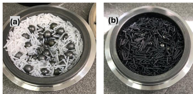
Figure 1. Photographs of PET-graphene mixtures in the milling jar: (a) before milling and (b) after milling.
