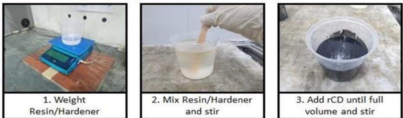
Figure 3. Schematic representation of the experimental methodology performed in this study
