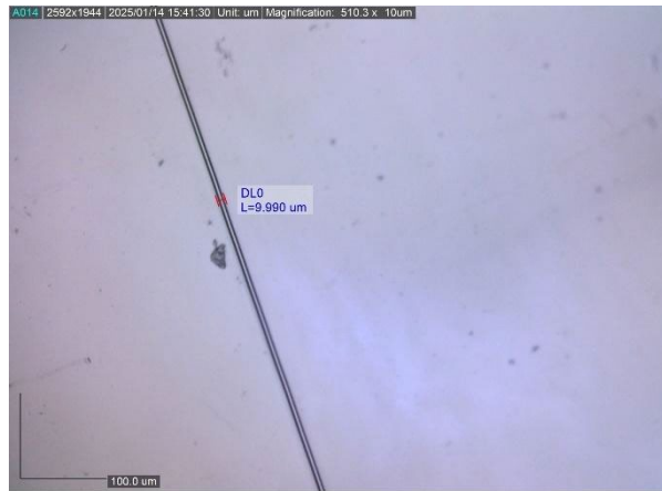
Figure 2. Dino Lite Microscope images for measuring 10 \mu\text{m} TOF.
