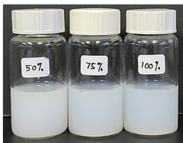
Figure 2. Visual appearance of lemon myrtle EO nanoemulsions prepared at different sonication amplitudes (50%, 75%, and 100%). Samples became less turbid as amplitude increased, reflecting smaller droplet size and improved optical clarity.
