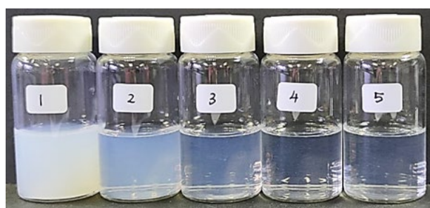
Figure 8. Photographic images of lemon myrtle EO nanoemulsions prepared with increasing surfactant concentrations (1–5% w/w). Samples transitioned from a cloudy/milky appearance to an optically transparent state as surfactant concentration increased.
