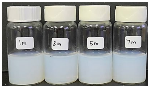
Figure 5. Visual appearance of lemon myrtle EO nanoemulsions prepared at different sonication times (1, 3, 5, and 7 minutes). Formulations appeared progressively clearer with longer sonication up to 5 minutes.
