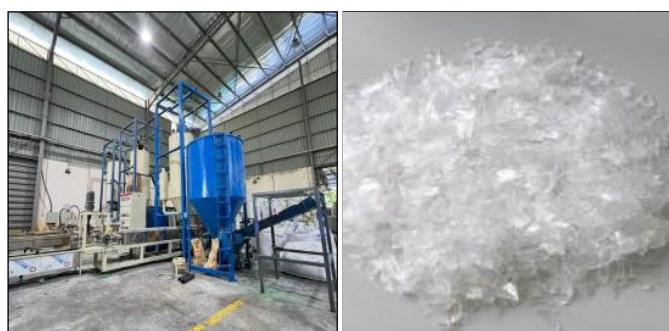
Figure 1. (a) PET recycling factory and (b) cleaned recycled PET flakes
