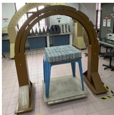
Figure 5. NRL Arch free space measuring equipment with PET-POFA composite brick specimens in vertical orientation
