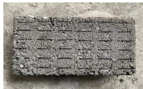
Figure 4. PET-POFA composite brick with surface slot array
