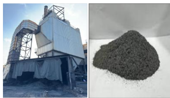
Figure 2. (a) Palm oil processing factory and (b) collected palm oil fuel ash (POFA) residue
