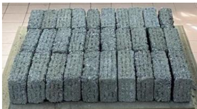
Figure 6. PET-POFA composite brick in vertical orientation
