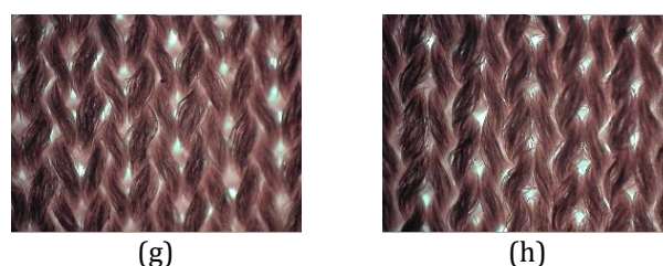
Figure 6. Microscopic views of IT fabric (g) face and (h) back
