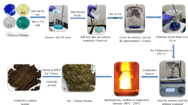
Figure 2. Schematic illustration of the solution combustion synthesis
