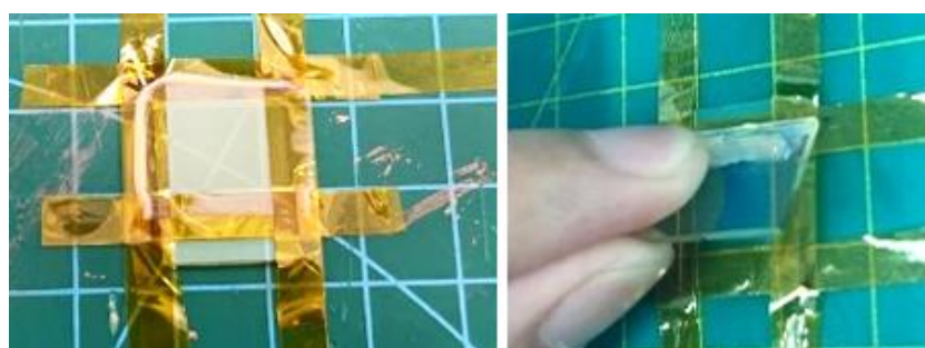
Figure 3. The TiO 2 paste was spread at 45-degree angle
