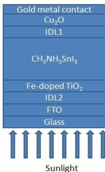
Figure 1. Simulated PSC using Fe-doped brookite TiO 2 as ETL
