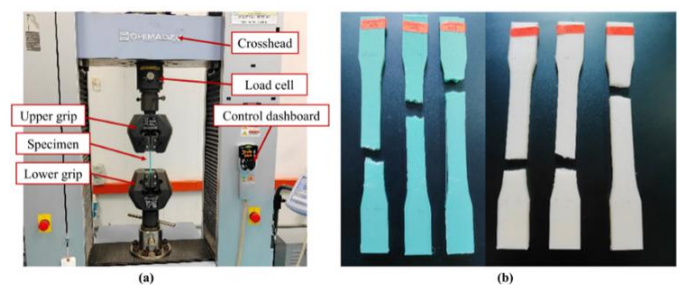
Figure 4. (a) Tensile testing setup using a Shimadzu Universal Testing Machine (b) Fractured 3D-printed PLA specimens after tensile testing
