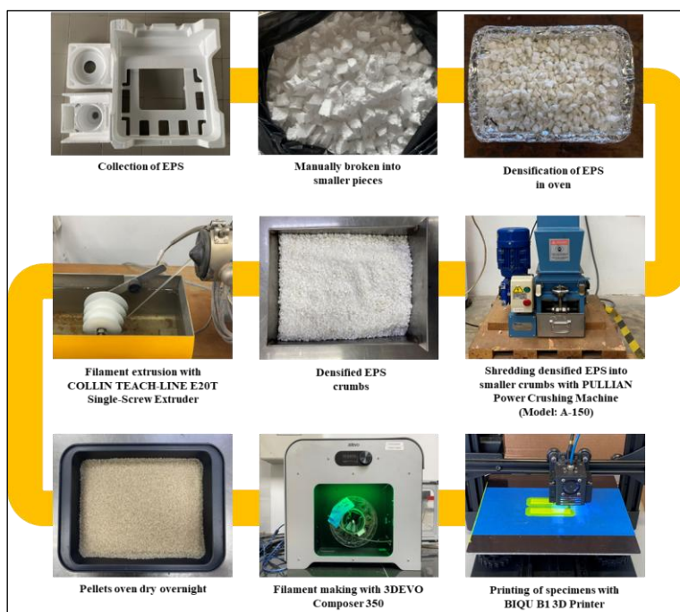
Figure 1. Process flow chart of printed specimens using rPS from EPS waste materials.
