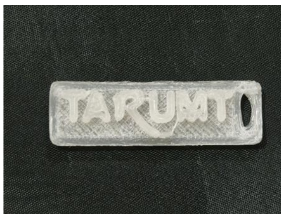
Figure 13. 3D printed TAR UMT keychain fabricated using filament made from a 50:50 rPP blend.
