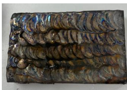
Figure 2. The nanocomposite coating sample on UNS S31803 grade steel plate with 50% overlapping weldment.
