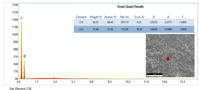
Figure 8. EDX analysis of the reduced graphene oxide
