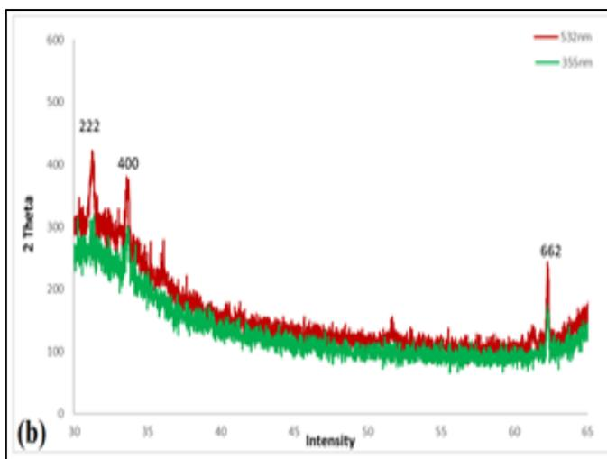
Figure 7. XRD patterns of In<sub>2</sub>O<sub>3</sub> at: a) three different laser wavelengths, b) two different laser wavelengths
