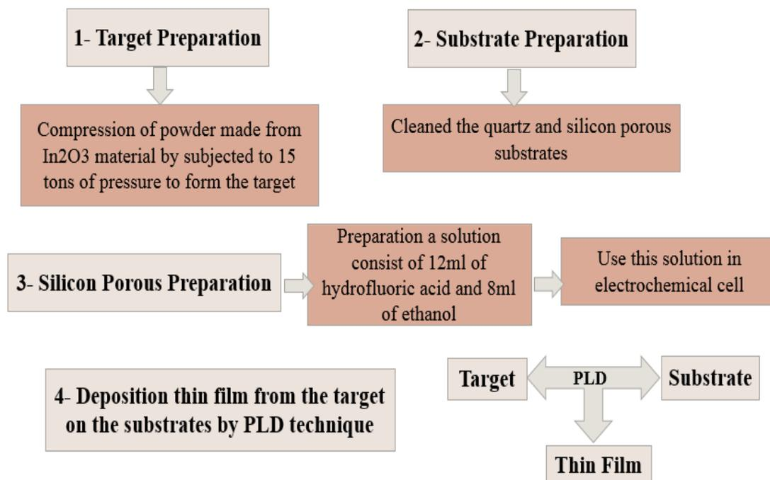
Figure 2. Flow chart of In<sub>2</sub>O<sub>3</sub> nanostructure thin film preparation process
