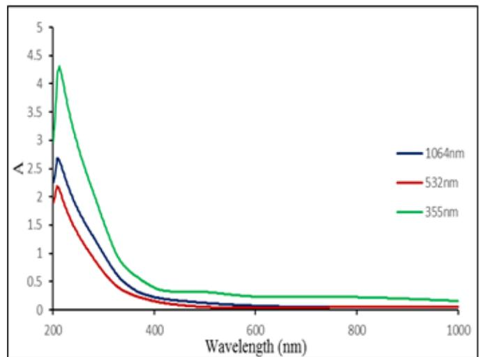
**Figure 4.** The-optical-absorption-of-  $\text{In}_2\text{O}_3$  at different-laser wavelength
