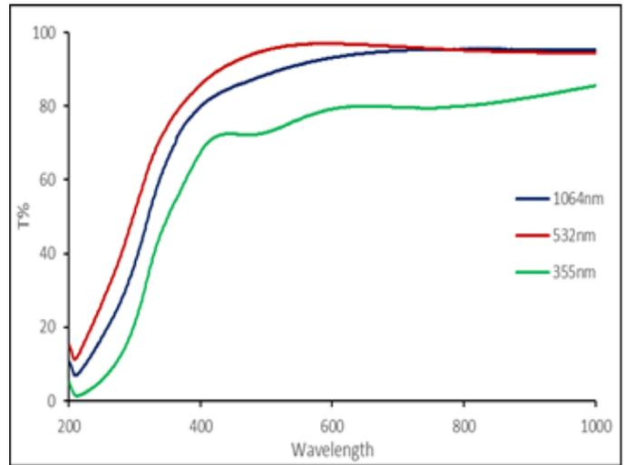
**Figure 3.** The-optical-transmission-of-  $\text{In}_2\text{O}_3$  at different-laser wavelength
