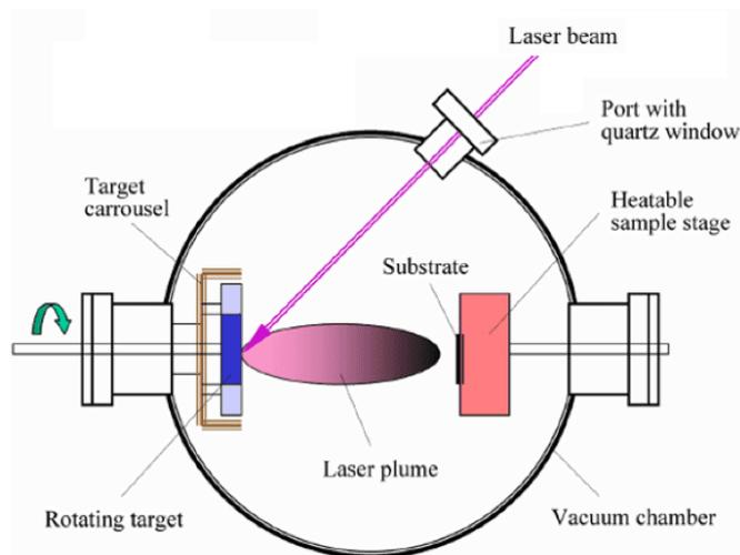
Figure 1. Deposition process by PLD
