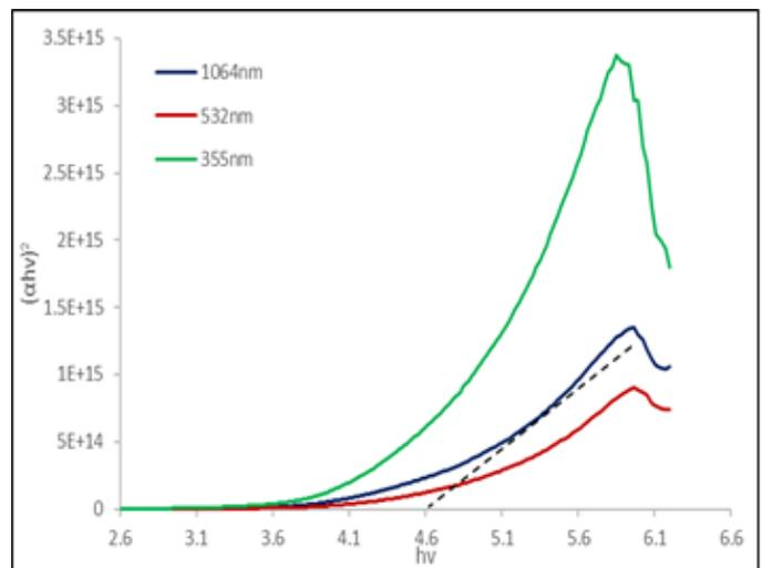
**Figure 5.** The optical band gap ( $E_g$ )-of-  $\text{In}_2\text{O}_3$  at different-laser wavelength
