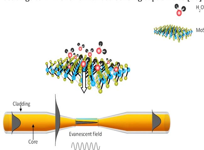
**Figure 1.** Interaction between the evanescent field of light and a TMF coated with  $\text{MoS}_2$ .
