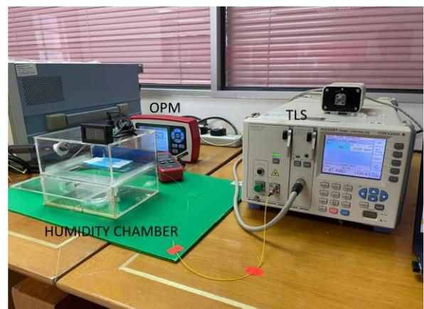
**Figure 4.** Experiment setup for sensing humidity
