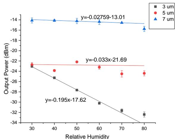
**Figure 6.** Humidity sensor performance by varying TMF size diameter
