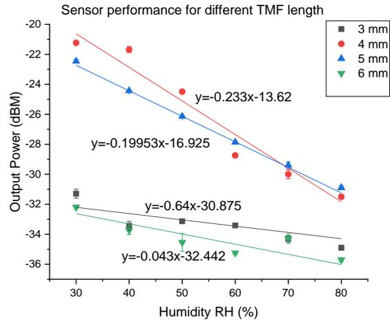
**Figure 5.** Humidity sensor for different tapered length fibre
