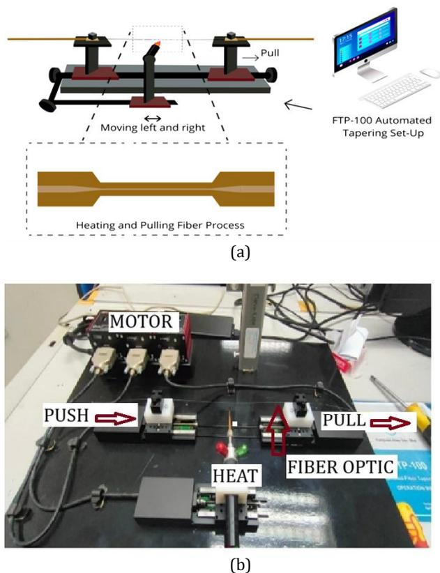
**Figure 2.** The tapered fibre optic for a (a) schematic and (b) actual setup
