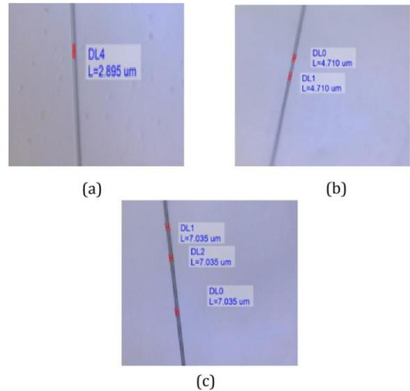
**Figure 3.** Dino Capture 2.0 images of the tapered optical fibre with size diameters approximately 3, 5 and 7  $\mu\text{m}$
