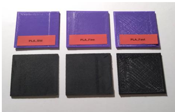
Figure 4 . 3D Printed substrates using standard PLA filament (purple) and enhanced-graphene PLA filament (black).
