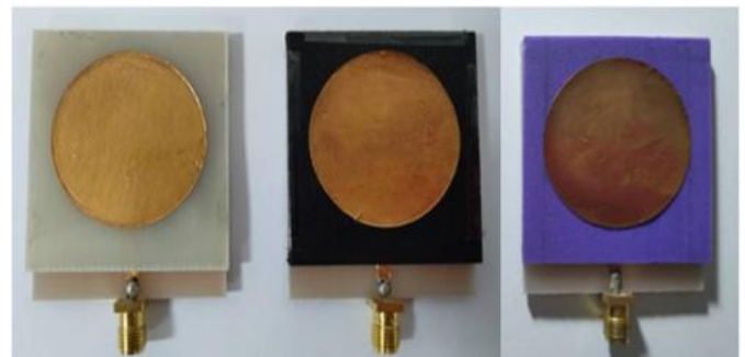
Figure 6. Prototypes of the proximity feed circular patch antenna. (left) FR-4 substrates upper and lower layers. (center) FR-4 substrate at lower layer and printed Enhanced-PLA Graphene at upper layer. (right) FR-4 substrate at lower layer and printed standard PLA at upper layer.
