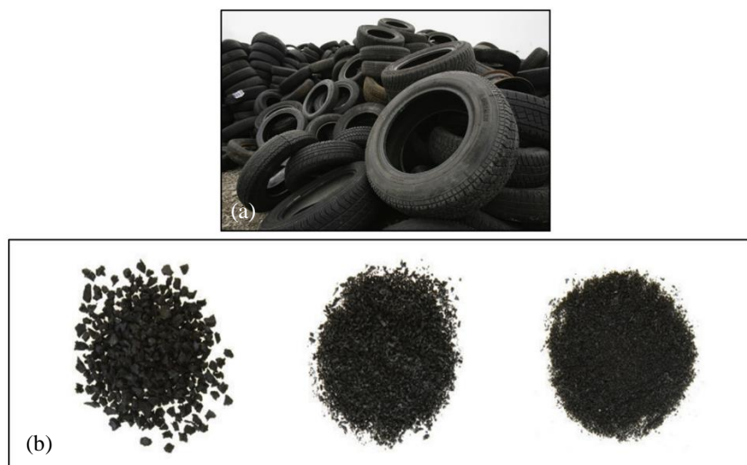
Figure 1 Waste tire products. (a) Stockpile of whole waste tires, (b) Tire derived products [5].
