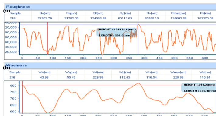
Figure 6. Surface roughness (a) and waviness (b) based on the black line showcased in the 2D image.
