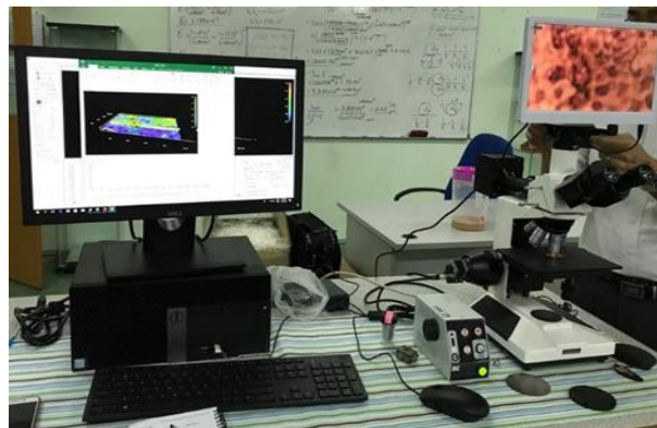
Figure 9. The 3D non-Contact Profilometer.
