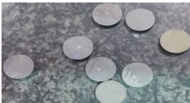
Figure 3. 22MnB5 Boron Steel with the shape of RNGN 120300 turning insert.
