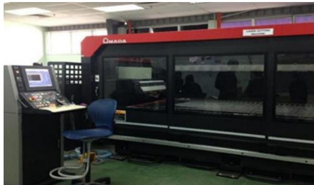
Figure 1. Laser facility employed to cut 22MnB5 Boron steel.
