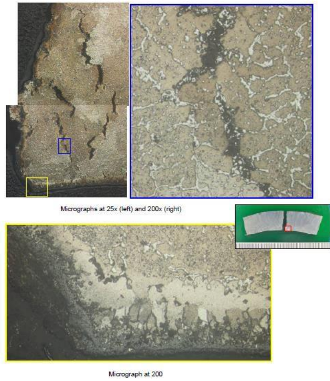
Figure 14. Metallographic Section of Tube A (Section #A) – Across Rupture Mouth (ID).
