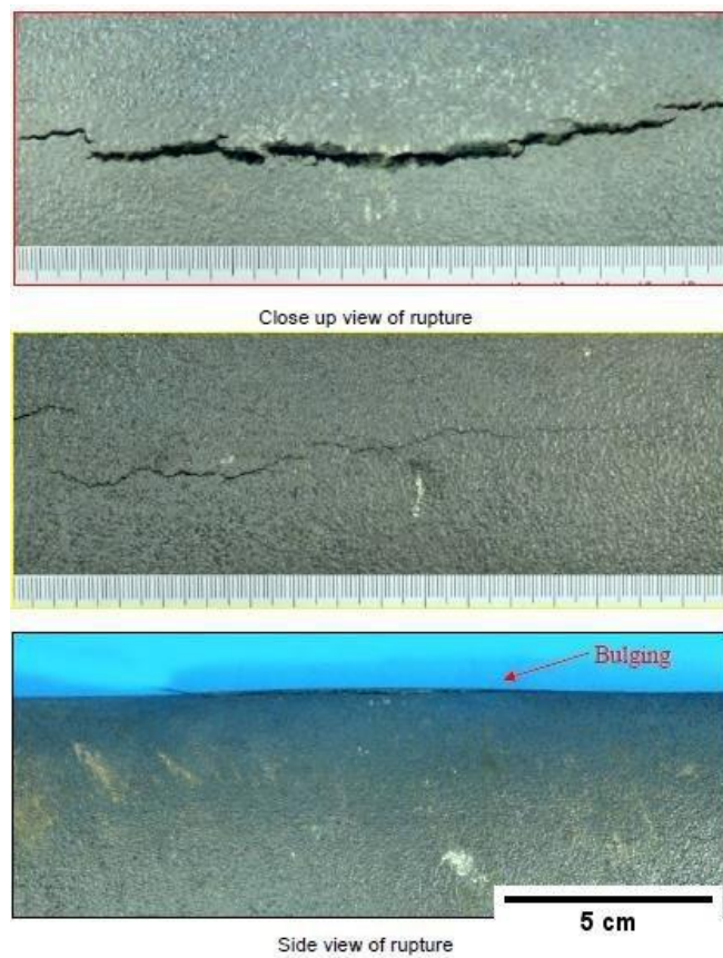
Figure 2. General Views of Tube A – OD Surface for both close-up and side views.
