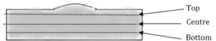
Figure 2. Depths of bead for micro-hardness measurement.
