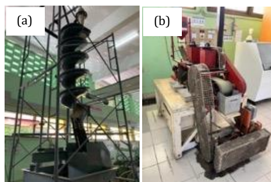
Figure 3. (a) Gravity separation via spiral and (b) magnetic separation via DDMS.
