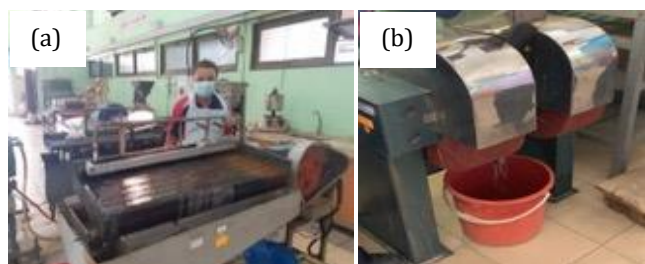
Figure 4. (a) Gravity separation via ST and (b) magnetic separation via WHIMS.
