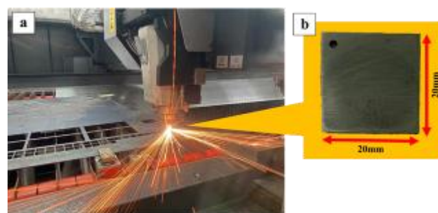
Figure 2. (a) Performing laser cutting to low carbon steel and (b) low carbon steel.
