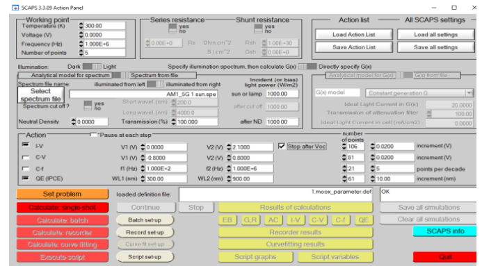
Figure 1. The SCAPs start-up panel or main panel.
