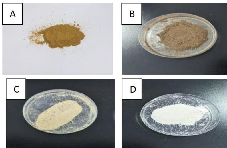
**Figure 2.** Photographs of ZnO NP powders with different calcine temperatures (a) shows the as-prepared sample and (b), (c), and (d) show samples calcined at 400, 600, and 800 °C, respectively.
