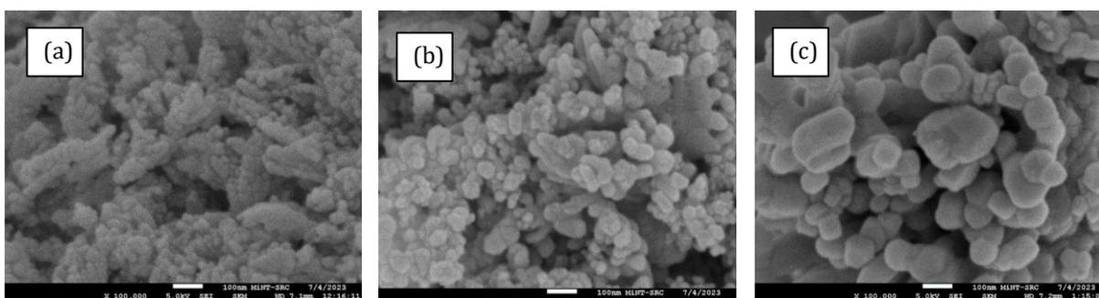
**Figure 4.** Microstructure analysis image of ZnO powders with different calcine temperatures at (a) 400, (b) 600, and (c) 800 °C, respectively.
