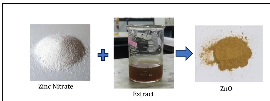
**Figure 1.** Schematic representation of ZnO NPs synthesis
