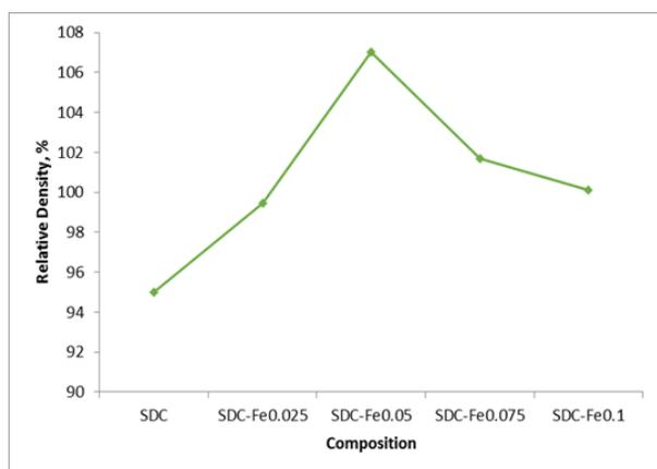
Figure 3. Density value sintered at 1480 °C.
