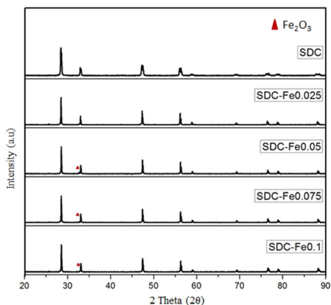
Figure 1. The diffractions peaks position with 2 theta degree.
