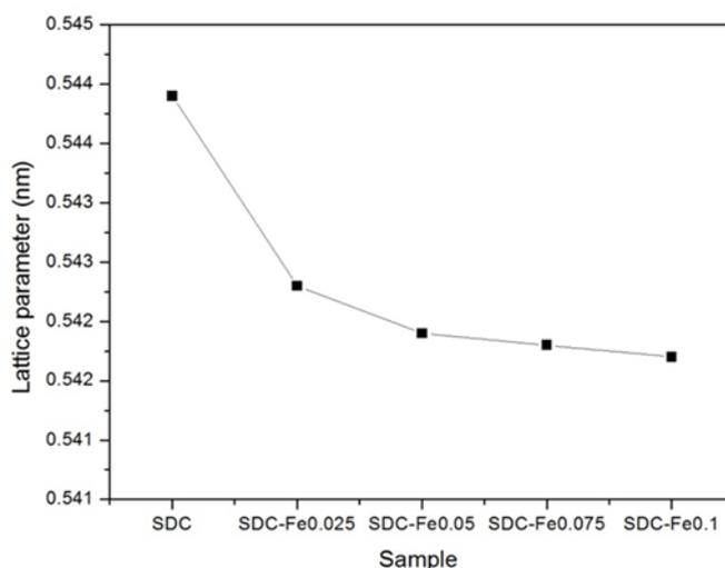
Figure 2. Lattice parameter of sample derived from XRD pattern.
