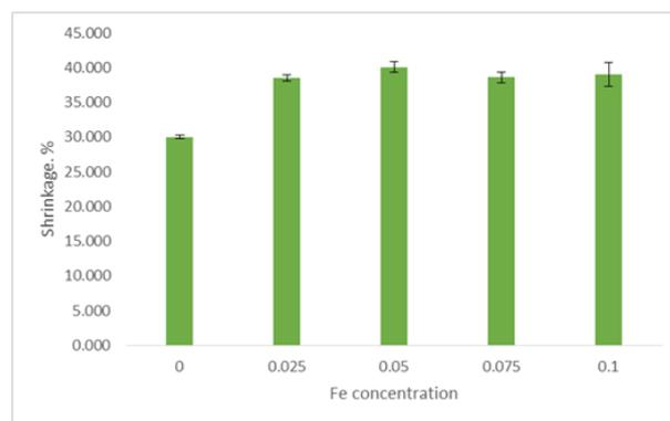
Figure 4. Volume shrinkage of sample sintered at 1480 °C.
