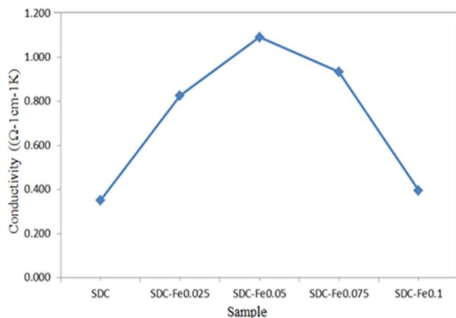
Figure 6. Total conductivity represent at 600 °C.
