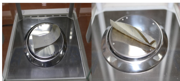
Figure 5. Folding of samples after exposure to manufacturing process residue chemicals except acetone and (b) Acetone
