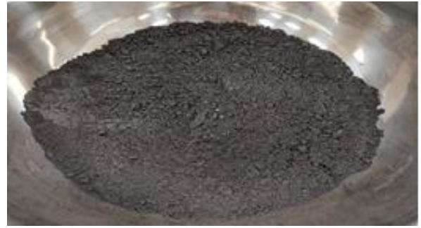
Figure 5. Bamboo biochar powder (BCP) sieved to 75 \mu m
