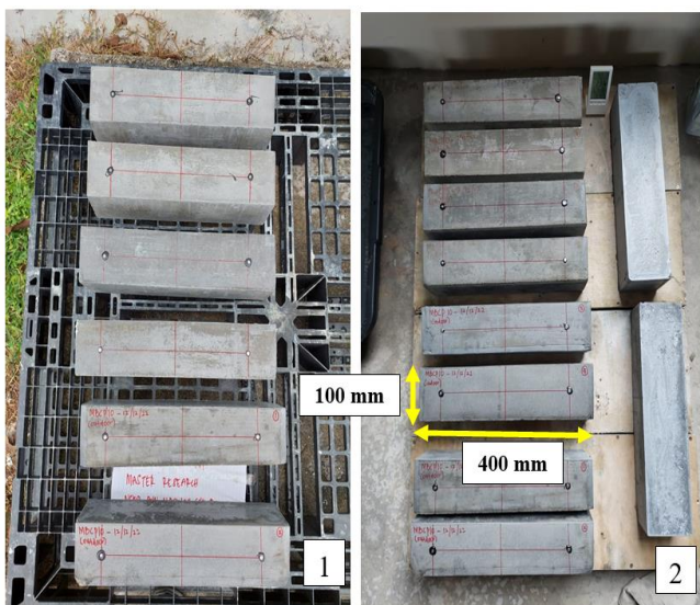
Figure 8. Hardened state of prisms mortar (1) outdoor, and (2) indoor conditions.
