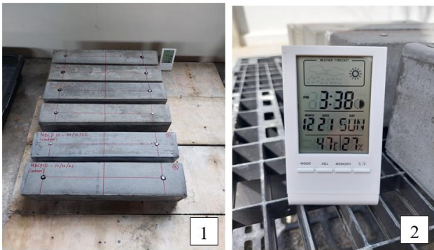
Figure 10. Measurement of relative humidity and temperature for (1) indoor and (2) outdoor exposure for 150 days study period by using a hygrometer
