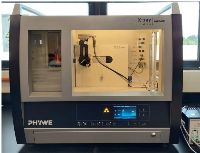
Figure 6. XRF analysis using Phywe XR 4.0 X-Ray instrument
