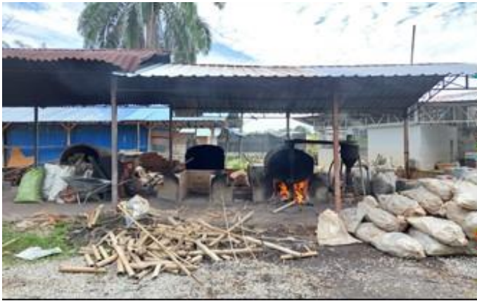
Figure 2. The slow pyrolysis process of bamboo waste to produce bamboo biochar was done at Tadam Hill Resorts, Selangor, Malaysia
