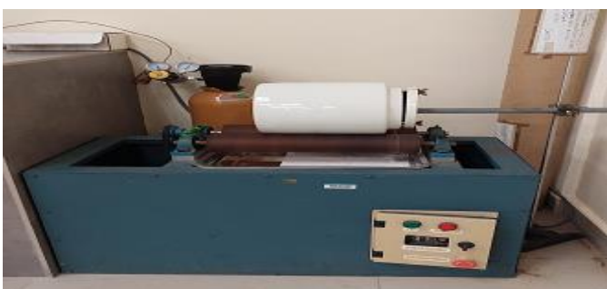
Figure 4. Laboratory ball mill machines used to grind bamboo biochar into powder size (75 microns)
