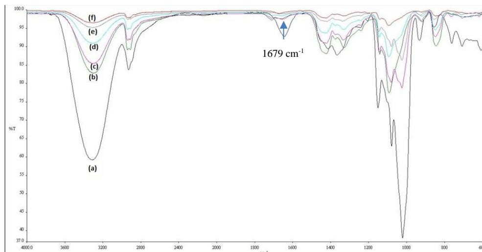
**Figure 5.** FTIR spectrum for (a) aloe vera extract powder; aloe vera’s content in the electrospun fibers (b) AV 0% w/w, (c) AV 5% w/w, (d) AV 25% w/w, (e) AV 50% w/w, (f) AV 75% w/w
