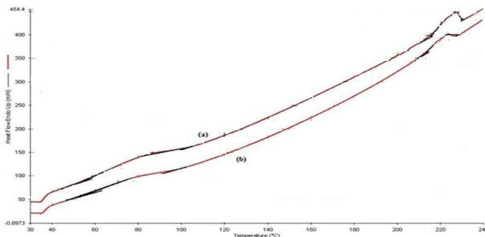
**Figure 6.** DSC thermograms for nanofibre of (a) electrospun PVA 100% and (b) electrospun PVA- aloe vera
