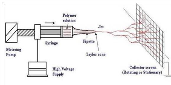
**Figure 2.** Schematic diagram of the electrospinning setup.
