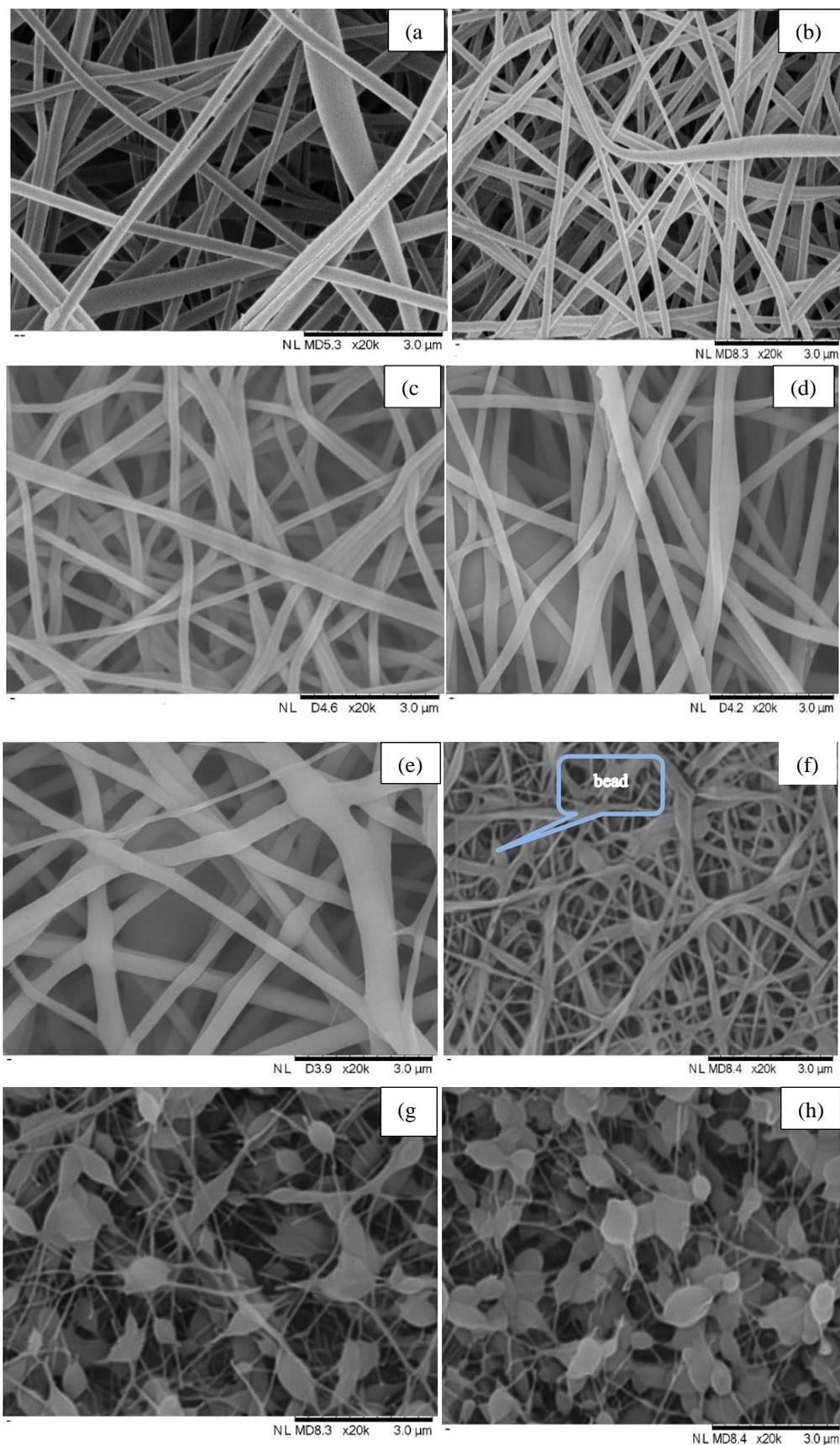
**Figure 4.** SEM micrograph of the electrospun aloe vera (AV)-PVA composite nanofibers; a) AV 0% w/w, b) AV 5% w/w, c) AV 10 %w/w, d) AV 15 %w/w, e) AV 20% w/w, f) AV 25% w/w, g) AV 50 % w/w and h) AV 75% w/w .
