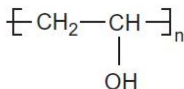
**Figure 1.** Chemical structure of Polyvinyl Alcohol (PVA).
