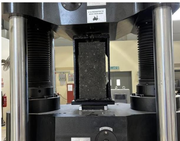
**Figure 6.** Pull-out test executed by using Universal Testing Machine (UTM)
