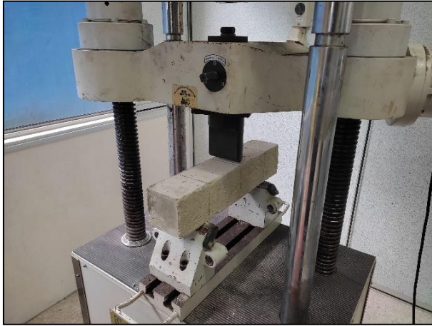
Fig. 5 – Flexural testing process
