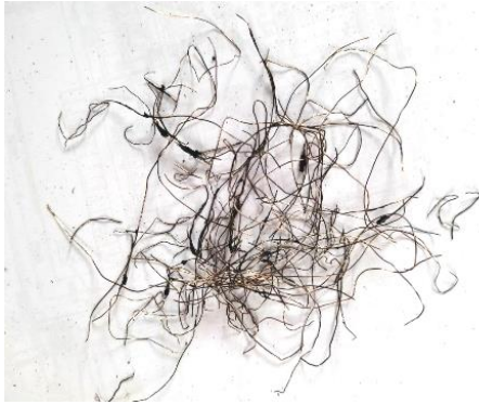
Fig. 3 – The selected SWW in diameter of 0.20 mm
