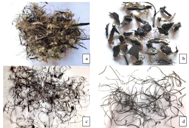
Fig. 1 – The SWW (a) original forms collected on site (b) rubber residue (c) steel wire with 0.2 mm diameter and (d) steel wire with a diameter 0.95 mm
