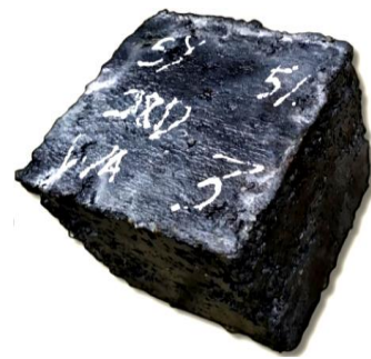
Fig. 10 – Physical appearance of concrete with SWW and CB addition
