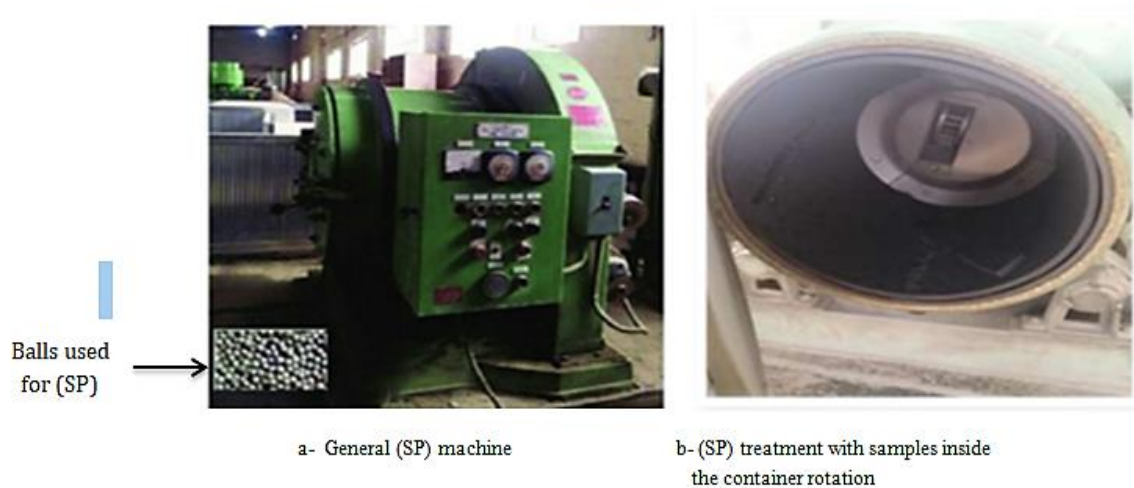
Figure 5. The shot peening device.
