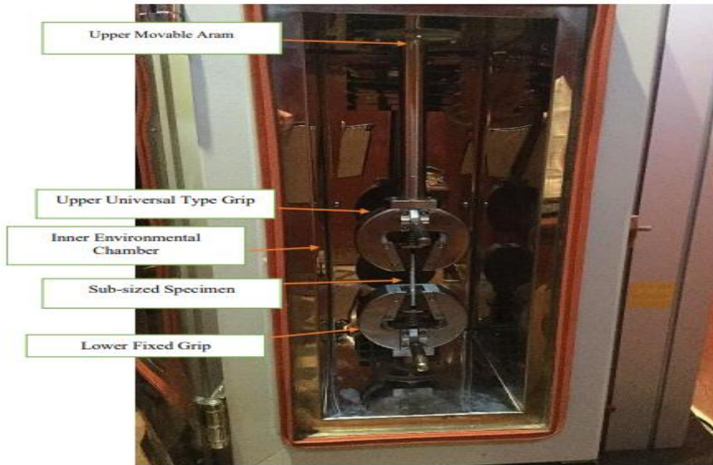
Figure 2. High-temperature tensile test specimen loaded into the grips with proper alignments.[17]
