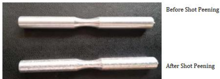
Figure 6. Specimens before and after shot peening.
