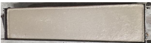
Figure 1 The slurry of raw materials in the box mold
