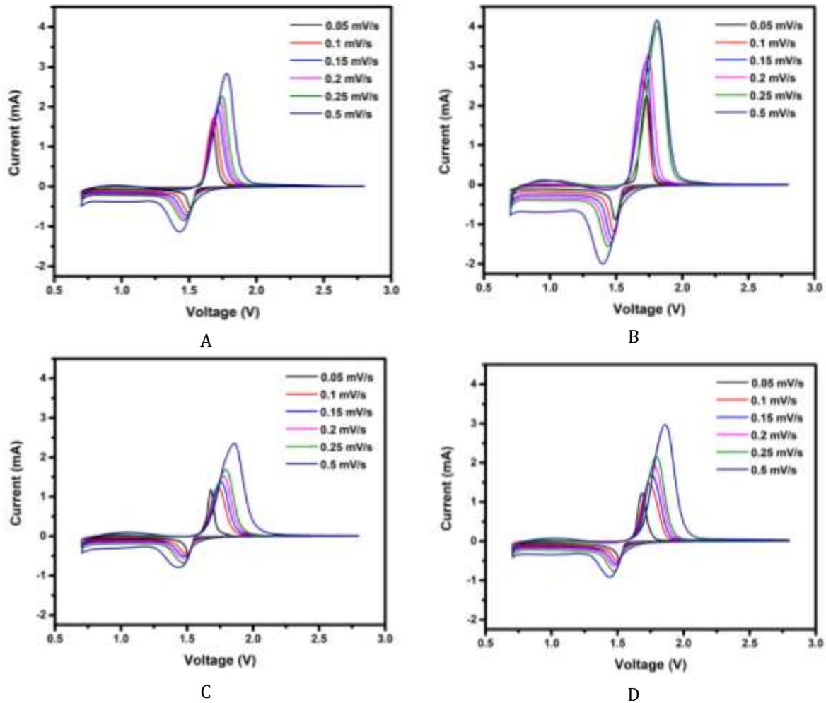
**Figure 7.** Cyclic voltammetry of: (A) Pure LTO, (B) LTO/SP, (C) LTO/Sugar, (D) LTO/SP+PVDF at different scan rates (0.05, 0.1, 0.15, 0.2, 0.25, and 0.5 mVs<sup>-1</sup>).
