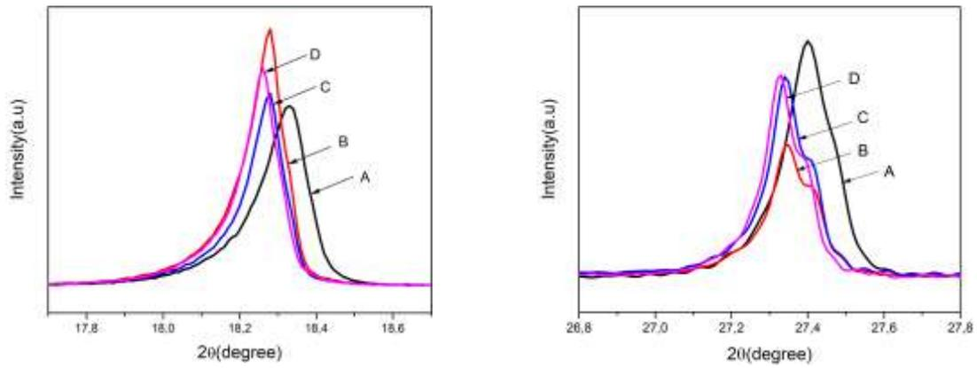
**Figure 2.** Detailed observation of [111] peak of LTO (left) and rutile (right) for: (A) Pure LTO, (B) LTO/SP, (C) LTO/Sugar, (D) LTO/SP+PVDF.
