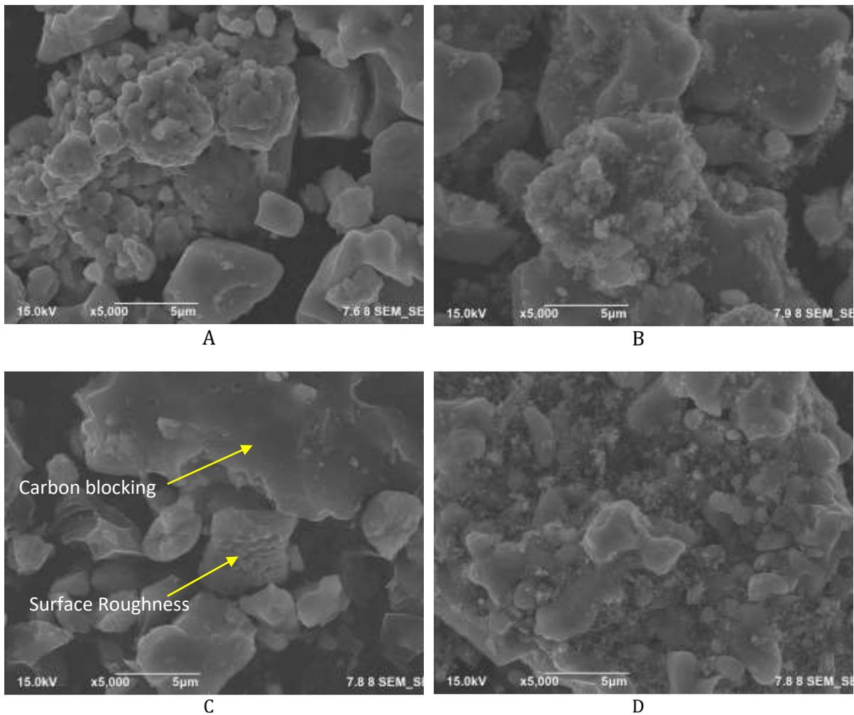
**Figure 3.** The FESEM images of: (A) Pure LTO, (B) LTO/SP, (C) LTO/Sugar, (D) LTO/SP+PVDF.
