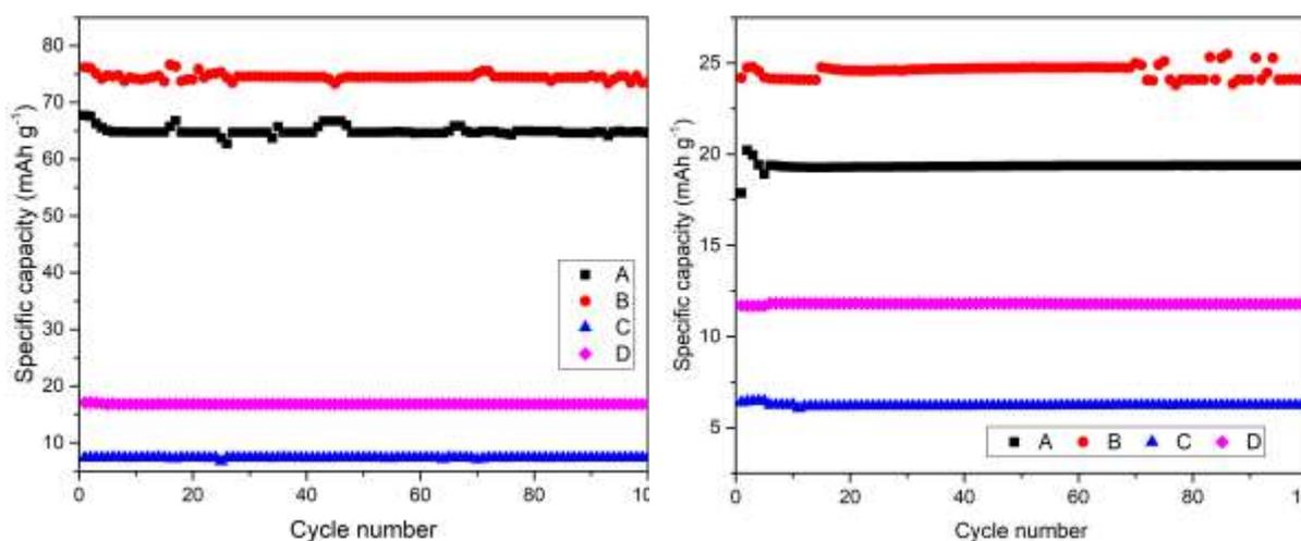
**Figure 11.** Cycling performance of: (A) Pure LTO, (B) LTO/SP, (C) LTO/Sugar, (D) LTO/SP+PVDF at (left) 5 C and (right) 10 C for 100 cycles.
