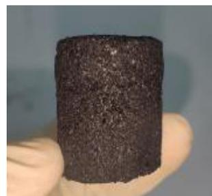
**Figure 2.** Solid fuel made from torrefied PKS mixed with HDPE.
