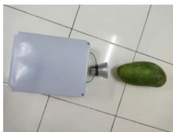
Figure 5. Ultrasound internal quality diagnostics device
