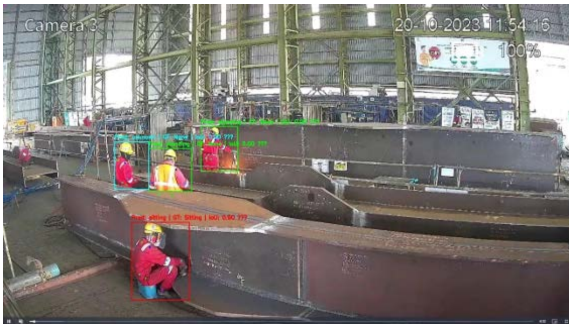
Figure 4. YOLOv8x-pose keypoint extraction and activity prediction result
