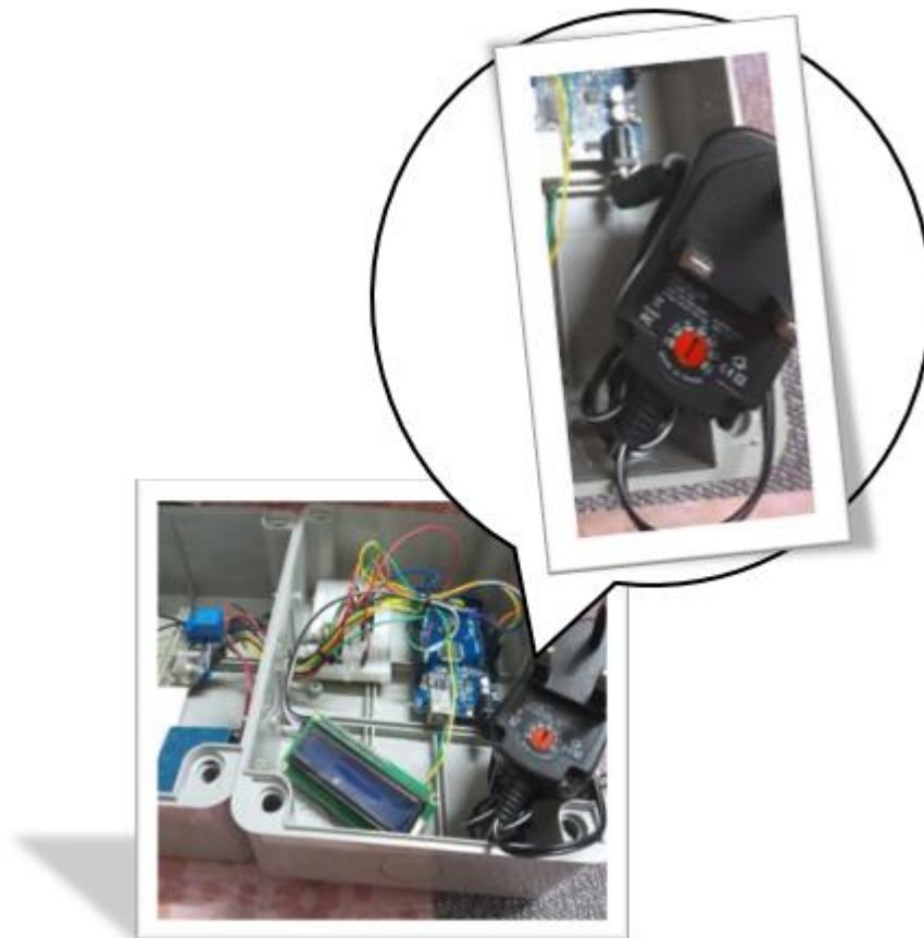
Figure 20: Utilizing a 6V DC Power Supply to Address Voltage Drops
