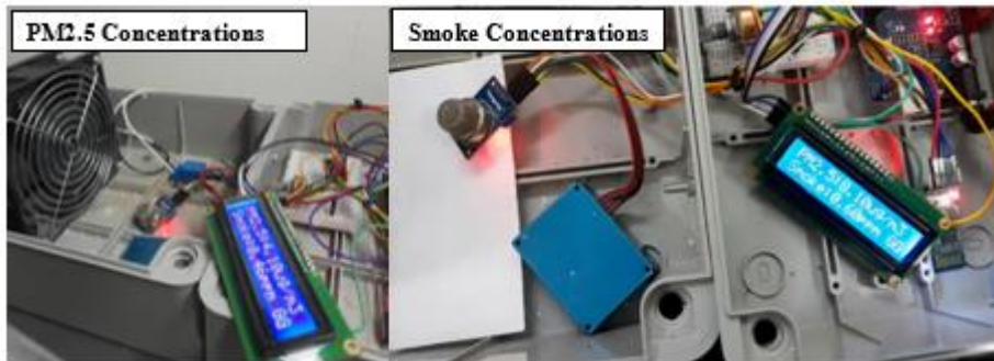
Figure 17(a): Sample 1 on AC Fan Remains Off in Response to Satisfactory Air Quality and Both Concentrations 'G' for Good
