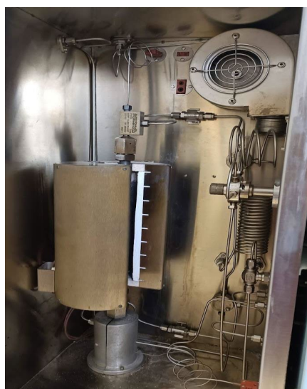
Figure 1: Reactor system for catalytic co-pyrolysis of cotton fabric waste and polypropylene plastic waste.
